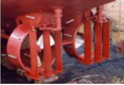
This deflection makes it possible for even large vessels and barge trains, like the *Island Monarch/Island Trader* ATB, to make tight turns. In trials, rudder side force is measured to be 74 percent of the bollard pull.
