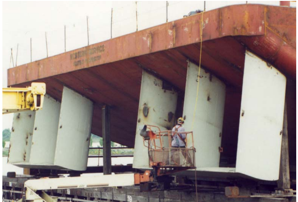
Invented by Joe Gruzling, President of NautiCAN Research more than 20 years ago, HYDRALIFT skegs add 10% or less resistance
