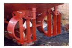
This deflection makes it possible for even large vessels and barge trains, like the *Island Monarch/Island Trader* ATB, to make tight turns. In trials, rudder side force is measured to be 74 percent of the bollard pull.
