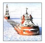
Robert Lemeur Arctic Class II icebreaker was built as 1/4 scale model of Arctic Pilot Project.
