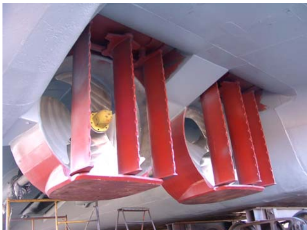
Figure 10. Edgar Kotokak after Refit with NautiCAN Nozzles
